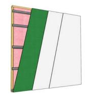
Type X Drywall 15.9 mm (5/8") Wood studs 50.9 mm x 101.6 mm (2" x 4") at 610 mm (24") c.c. R-12 Batt Insulation Resilient channel at 610 mm (24") c.c. **SONOpan** 19 mm (3/4") Type X Drywall 15.9 mm (5/8") Type X Drywall 15.9 mm (5/8")
