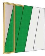
Type X Drywall 15.9 mm (5/8") **SONOpan** 19 mm (3/4") Wood studs 50.9 mm x 139.7 mm (2 "x 6") at 610 mm (24") c.c. **SONOpan** 19 mm (3/4") Type X Drywall 15.9 mm (5/8") Type X Drywall 15.9 mm (5/8")
