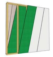
Type X Drywall 15.9 mm (5/8") Type X Drywall 15.9 mm (5/8") **SONOpan** 19 mm (3/4") Wood studs 50.9 mm x 139.7 mm (2 "x 6") at 610 mm (24") c.c. **SONOpan** 19 mm (3/4") Type X Drywall 15.9 mm (5/8") Type X Drywall 15.9 mm (5/8")
